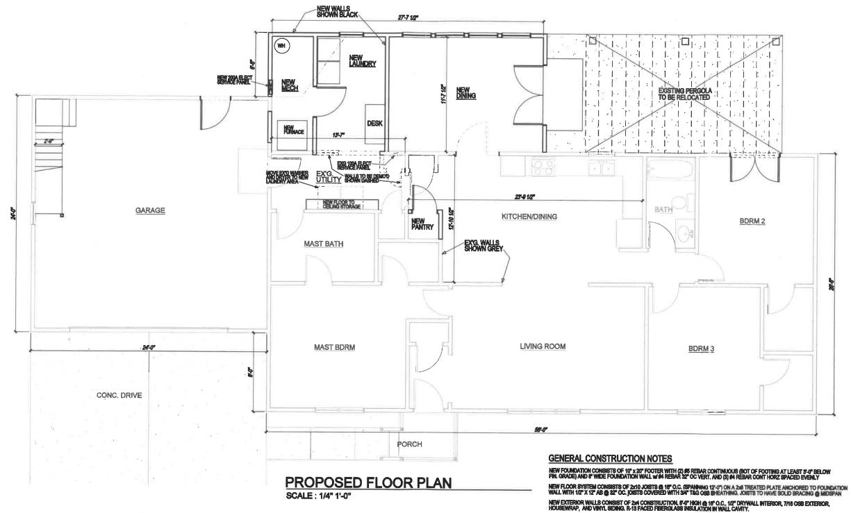
NEW INTERIOR WALLS CONSIST OF 2x4 CONSTRUCTION, 8-0" HIGH  $\underline{\mathbf{0}}$  18" O.C., 12" DRYWALL BOTH SIDES
